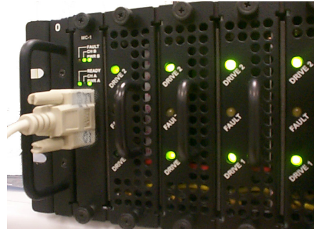
Exhibit 7-1: The management card may be accessed via a serial port DB-9 connector or an optional Ethernet connection.
